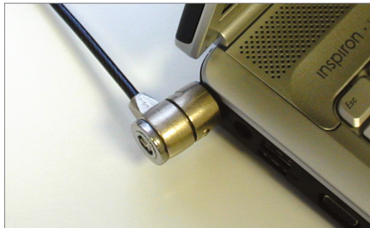
FIGURE 10.3 A laptop security cable
