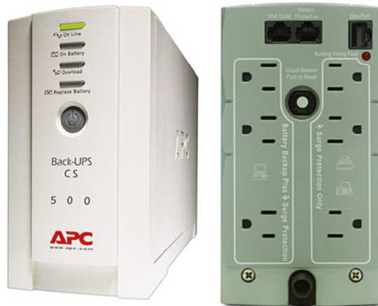
FIGURE 12.2 Front and back of a UPS
