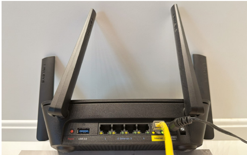
FIGURE 8.8 A wireless router
