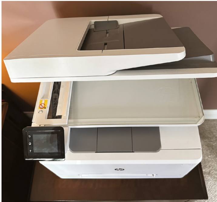
FIGURE 2.44 Laser printer with lid ajar to reveal scanning glass
