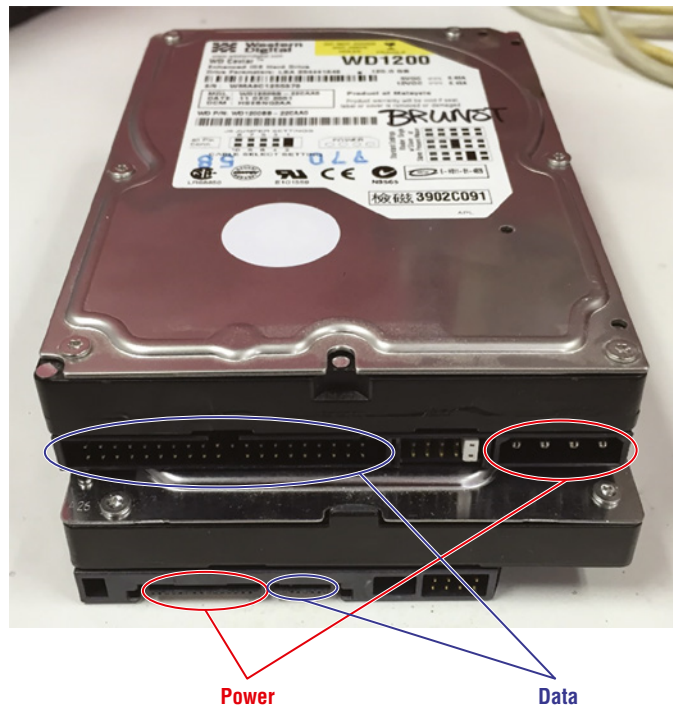
FIGURE 1.21 PATA/IDE and SATA hard drives
