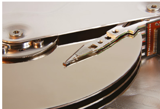
FIGURE 1.20 Inside a hard drive
