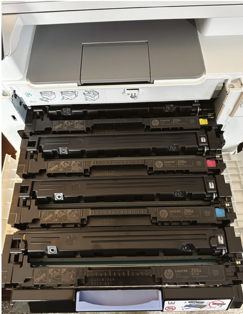
FIGURE 2.43 Laser printer toner cartridges in a printer
