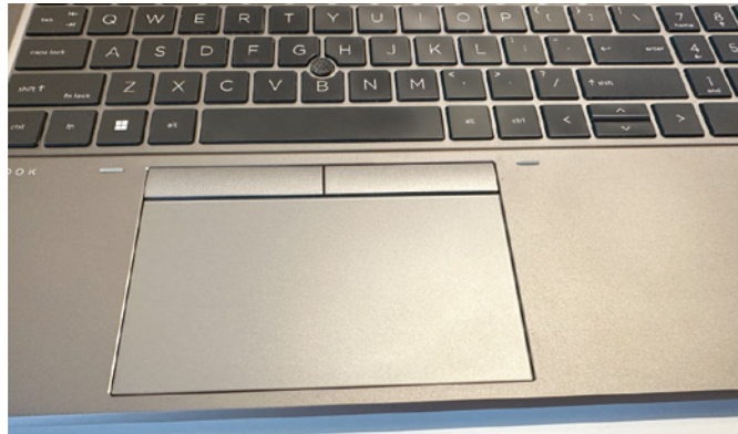
FIGURE 3.7 Point stick and touchpad on a laptop
