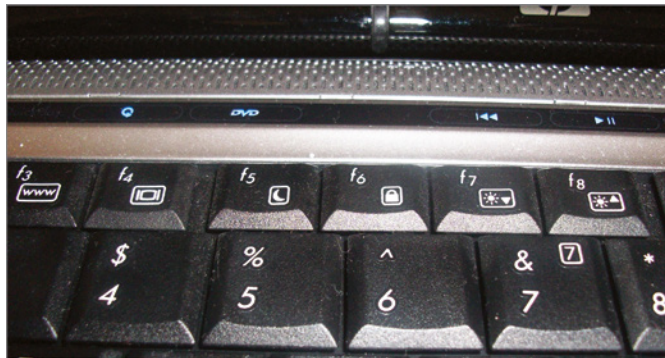
FIGURE 2.10 Video adjustment keys including F4 (LCD toggle), F7 (dim), and F8 (brighten)
